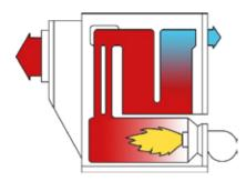
In a cylindrical furnance the flame burns freely in the middle and heats evenly. Furnance is made of high quality special steel, which temperature level of peeling is 1050°C.
