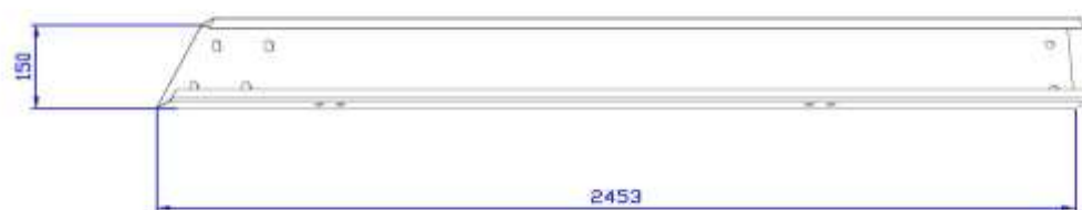
122055 INTERMEDIATE SUPPORT 1 T30 L=2453 mm
