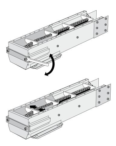
11. NB! Fit inlet/outlet with existing bolts.
