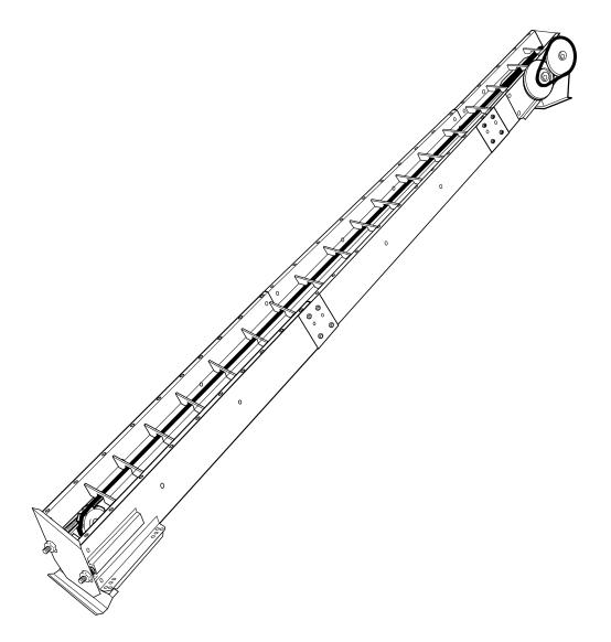
Tighten the conveyor chain with the tensioning bolts in the tail end.
