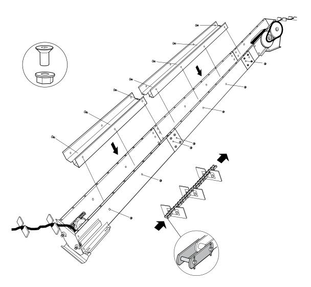
Lay the rest of the conveyor chain on the upper level.
