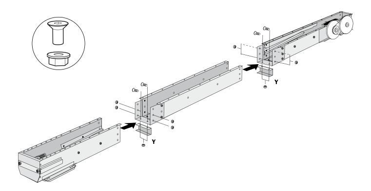
4. Assemble the lengths of chain into one long conveyor chain.
