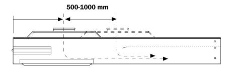
Inlets can also be located further in toward the intermediate section if a tail end with raised lid is used. See illustrated dimensions.
