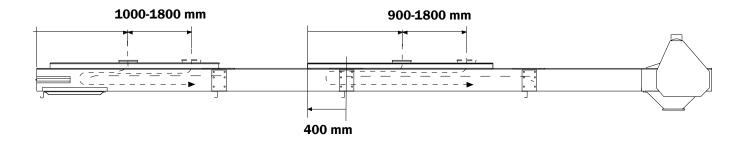
Side inletSide inlets are self-regulating and used for feeding from a silo/ storage bin.
