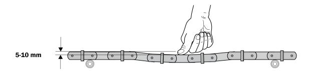
The following applies if the conveyor does not have intermediate sections with tensioning pulleys:
