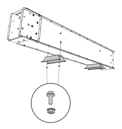
Fit guide plates in the sections with intermediate tray.
