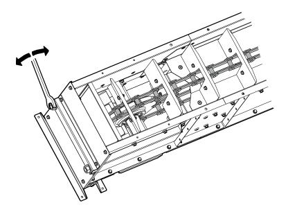
Check the tension of the conveyor chain by pressing it down between the two return rollers. If it can be pressed down 5-10 mm it is tensioned correctly.
