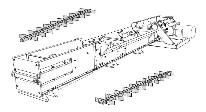
Tighten the conveyor chain with the tensioning bolts in the tail end.
