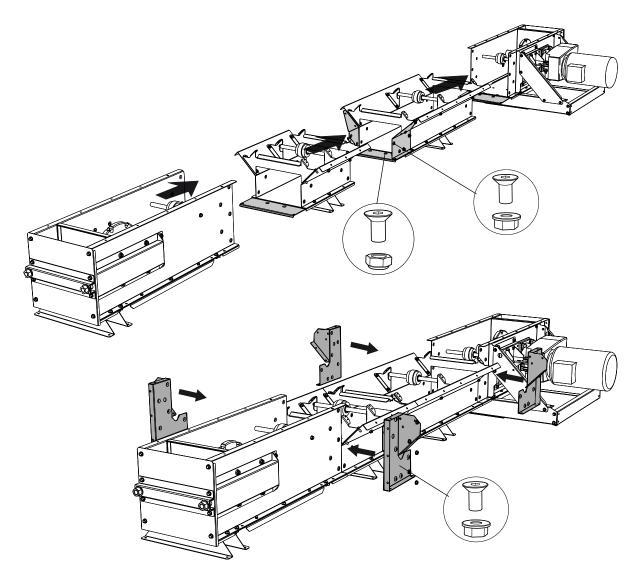
4. Fit the chain return rollers in the intermediate sections.
