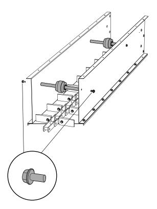
Assemble the lengths of chain in the bottom of the conveyor.
