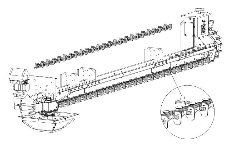
Tighten the conveyor chain with the tensioning bolts in the drive end.
