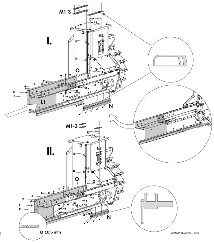
5. Assemble the machine parts (A, K1-2, L) with joint parts (H, I), bolt unions and brace rails (J) in accordance with the illustration.
