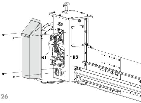
Holes for fitting electrical connection components and routing-through of cables are located on the drive end's frame plate (A).
