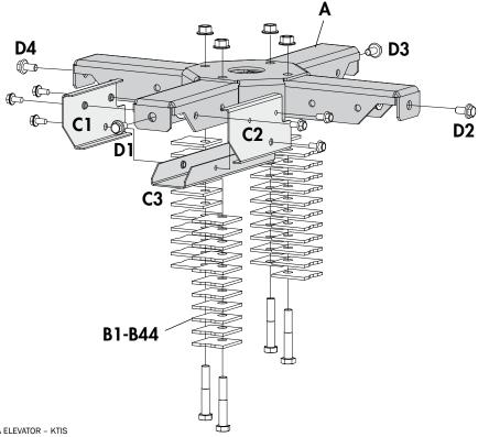
2. Fit the centre outlet cross (A) in the centre outlet hopper (E) with bolt unions (D1-D4).
