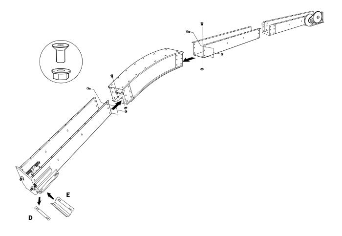
Assemble the lengths of chain into one long conveyor chain.
