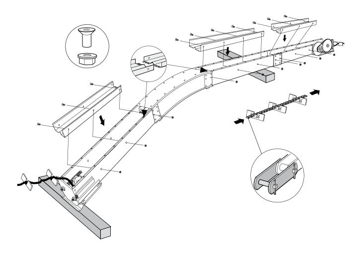
Lay the rest of the conveyor chain on the upper level.
