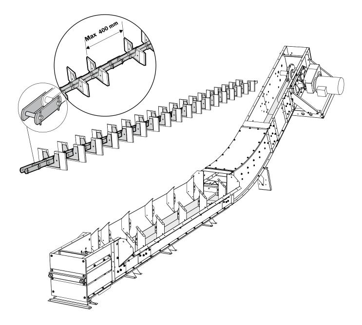
Fit the intermediate trays from the bend and outwards.
