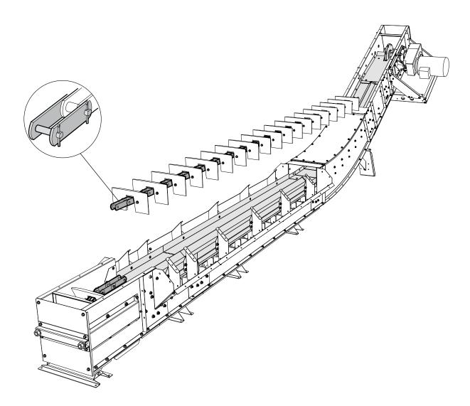
Tighten the conveyor chain with the tensioning bolts in the tail end.
