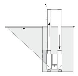
If the intake pit directs the flow 90° from the bucket belt, the connection is to be done via an extended inlet hopper (B).
