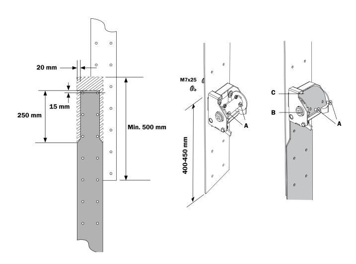
Mount the belt tensioner about 400-450 mm up on the end of the belt pointing downward.
