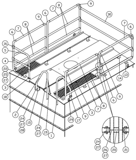
The figure shows the roof railings of the mobile dryer. Note the lifting lugs (29).
