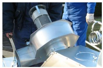
The aspirator is connected to the rear socket of the mobile dryer, which serves as the power source (see section 3.9). Hang the cable onto the brackets running along the elevator.
