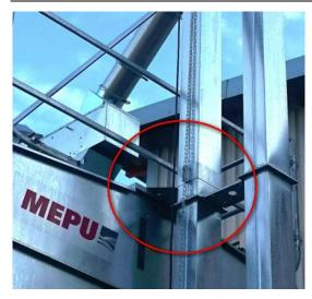
Check that the elevator is in a straight position (if necessary, check with an angle level and a spirit level). Tighten all connections carefully.
