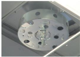
Connect the divider's changeover sleeve to the divider. Note that the orifice of the sleeve must be on the same side as the divider's operating lever (i.e. at the elevator's side). Use hex screws M6x16.
