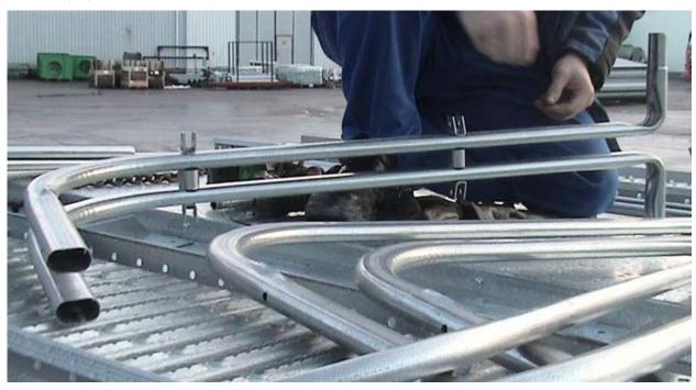
The side railings running lengthwise in respect to the mobile dryer consist of two railing elements, which are attached to the roof bridge with M8x75 hex screws and 26x48 mm washers. The railing elements are built using the parts assembled at the preceding stage and parts 6, 7, 8 and 9.
