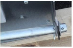
Push the guide bar through the sleeve of the articulation from the desired direction, and lock with cotter pins, do not forget to use washers on both sides.
