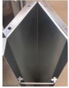
The so-called reinforced drying cell will be installed in the uppermost position. This drying cell can be identified by the reinforcement in the lower edge of the ridge, cf. the above photograph.
