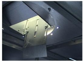
Fasten the shaft (14) to the worm gear motor (21) with hex screws M8x20 and a wedge 8x40. Mount the spreader disk (13) inside the grain bin with hex screws M8x16 and tighten with nuts. You can preadjust the spreader disc such that the holes in its bottom seem round. More detailed instructions can be found in the operating manual.
