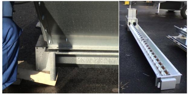
Connect the plug of the rotation sensor at the end of the bottom auger into the rectangular socket under the furnace. If the bottom auger is equipped with its own motor, the auger's power cable should also be connected, and the plug of the rotation sensor from the elevator is connected to its own socket.
