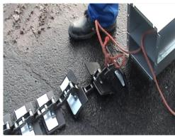
When the chain has reached the shaft at the top of the elevator, you can ease the advancing of the chain in the elevator by rotating the shaft at the top end. Remove the rope only after the chain is situated in both tubes all the way from top to bottom.
