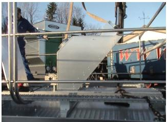
First remove the rain cover in the middle of the roof, which covers the hole for the precleaner. After that, attach the pre-cleaner loosely with hex screws M8x20, washers on both sides. Tighten the seams to prevent leaks with Butyl mastic between the edges.
