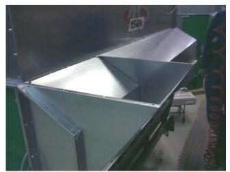
Fasten the end plates on top of the channel with hex screws M8x16.
