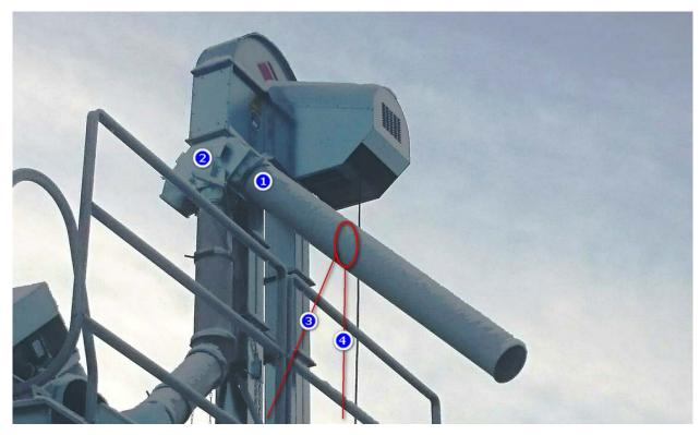
Grain unloading pipes (part 1) must be supported sufficiently, so that the divider (part 2) would not become bent.
