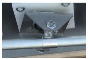
Fasten the articulation of the guide bar into the eye of the bearing at the end of the feeding auger.
