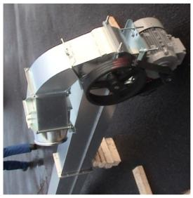
Connect the divider and the pre-cleaner. Use for connection a  $\emptyset 200$  mm stainless steel telescope pipe, which is attached at the top end with a  $15^{\circ}$  cast bend, and at the bottom end with a  $7^{\circ}$  cast bend to the pre-cleaners coupling (8). Mount the inner pipe to the pre-cleaner and the outer pipe on the top of the elevator and fasten to the divider. Make sure to install the dust seal on top of the inner pipe and tighten with a quick tie.
