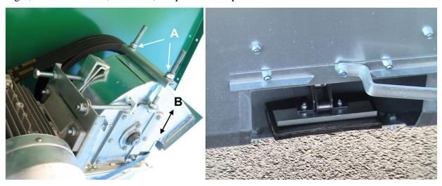
The tightening nuts for tightening the elevator chain (A), and the place to measure the distance (B).
