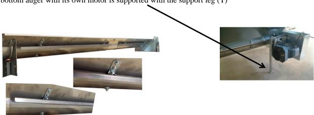
The bottom auger is fitted with a hatch, which makes it easier to clean the equipment, e.g. when drying seed grain. It is forbidden to open the hatches when the dryer is in use.
