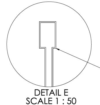
50mm ledge all the way around the auger trench for the lid to rest on. The ledge has to be as deep as the lid is thick.
