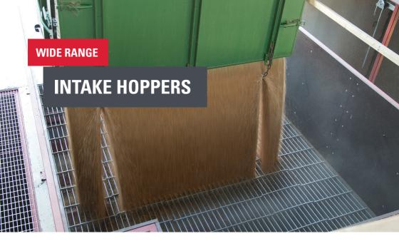
The Mepu range includes small and large hoppers to meet the needs of all customers. We offer drive-over hoppers, self-supporting hoppers equipped with chain conveyor, and traditional intake pits for dryer houses. The hoppers are assembled using bolted joints.
