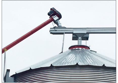
200mm/250mm pipe connection to the discharge end
