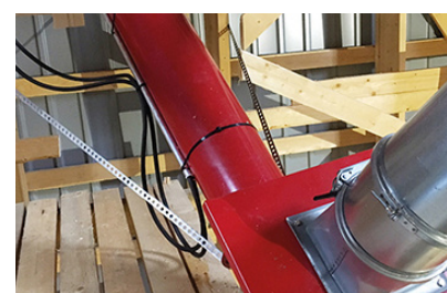
Hopper / 160mm/200mm pipe connection to the hopper
