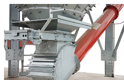
Inlet with 5° notches / Knife shutter
