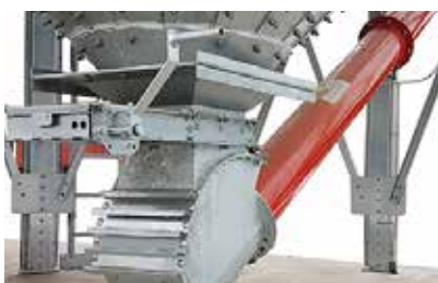
Inlet with 5° notches / Knife shutter
