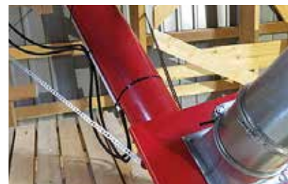
Hopper / 160mm/200mm pipe connection to the hopper
