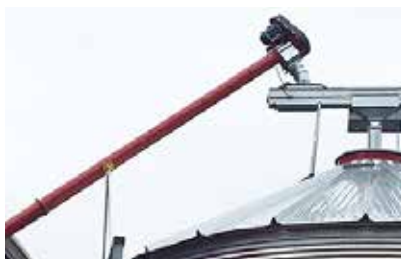
200mm/250mm pipe connection to the discharge end
